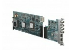
NXLK-IP40F SDI-IP converter board with 3G-SDI and SFP+ ports
