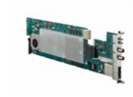
NXLK-IP51Y 12G SDI-IP Converter Board with two 1.5/3G-SDI and two 12G-SDI ports, supporting SMPTE ST 2110 in HD/4K and HDR
