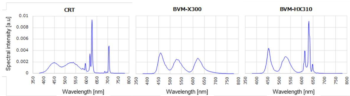
Figure 1. Spectrum of CRT, BVM-X300 and BVM-HX310
