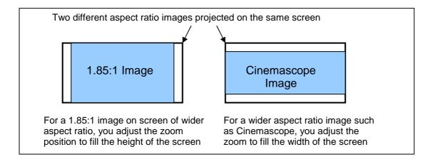
During the installation procedure Zoom and Focus are manually adjusted for each of the image framing positions and the Zoom/Focus positions are memorised for each aspect ratio setting by saving them in the Function Memory. During operation the lens can switch between different aspect ratios by recalling the appropriate Function memory setting.
