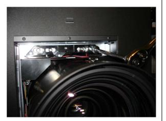
2. Connect the three cable harnesses; Focus, Zoom and Potentio; to their respective connectors on the projector chassis.
