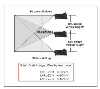
V shift is adjusted using a manual knob located above the lens mount mechanism.
